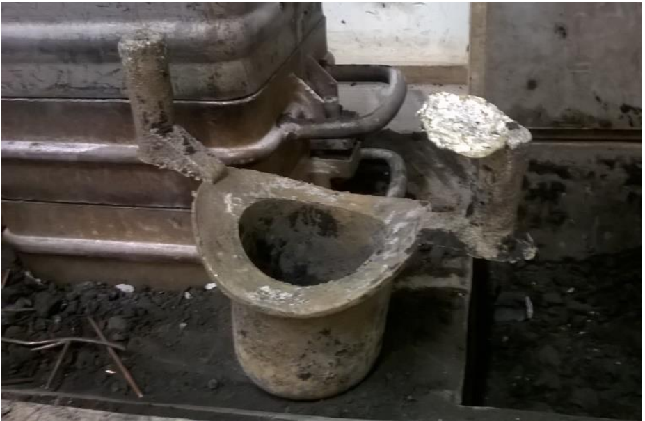
Cast Dome riser and pourer still attached
