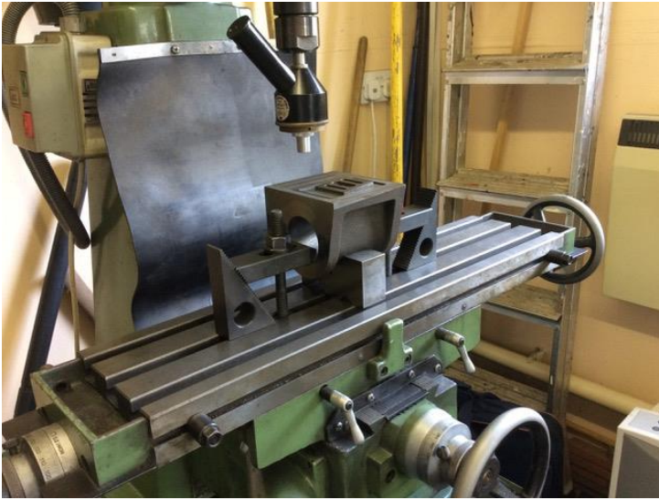
Lining up the edge using Optiset with 25x magnification
