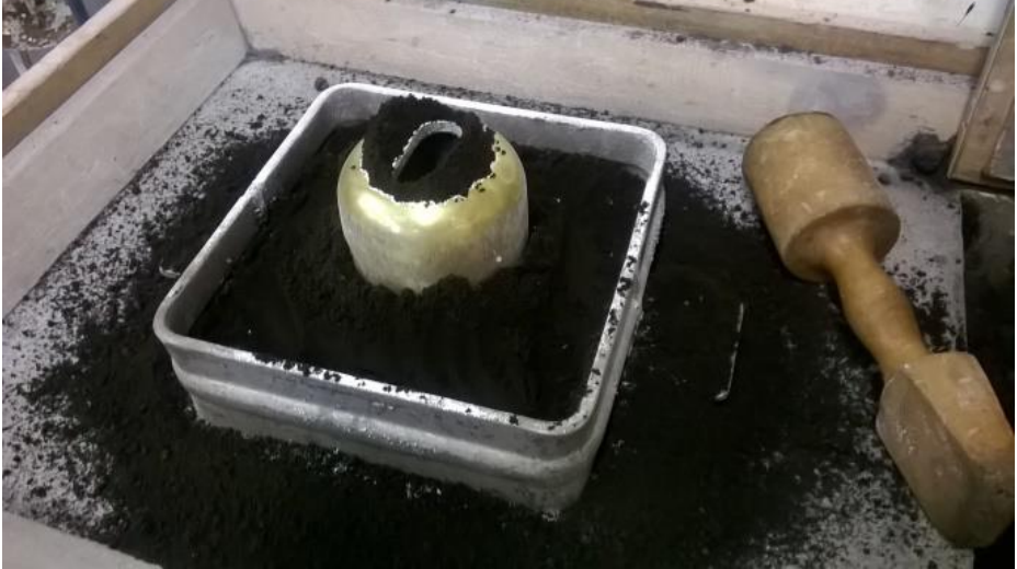
Sand box (Drag) with sieved sand ready for compacting, then extending with a second Pair of boxes
