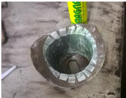
Existing Dome in use as a pattern
