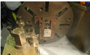
3. Axlebox jig mounted to centre the first box
