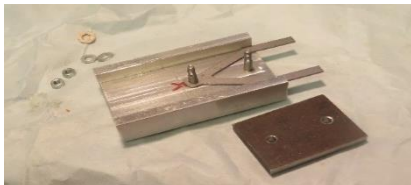
9. Bending jig stage 1
