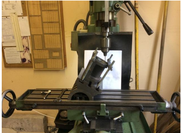
Drilling the drain cocks
