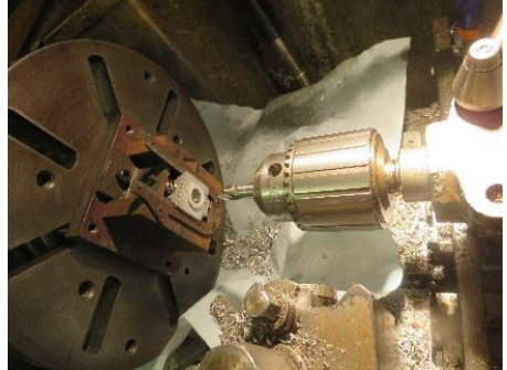
5. Opening up the bore
