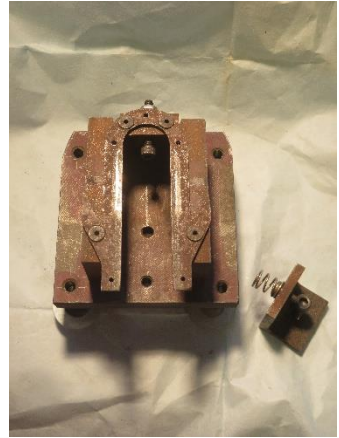
2. Axlebox machining jig
