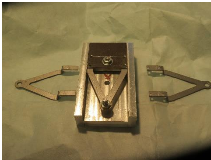
15. Set to drill the bent hangers
