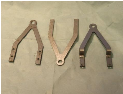
8. A pair of finished hangers with laser cut blank
