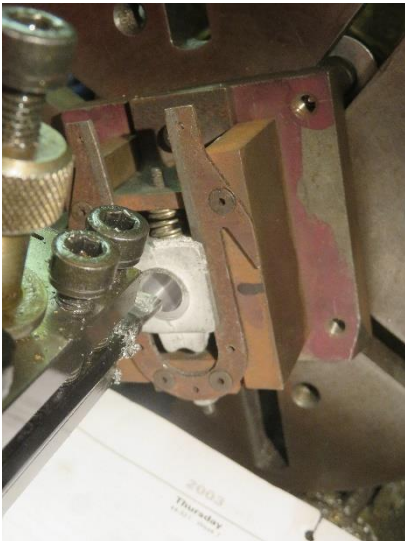
6. Final boring of a box
