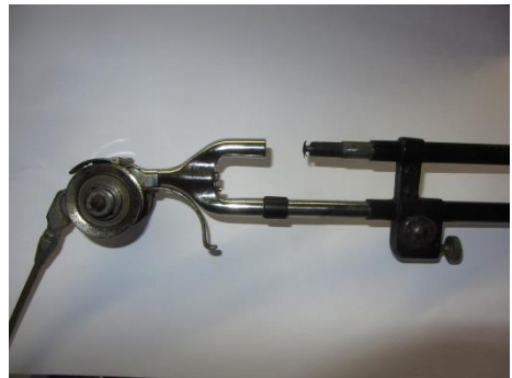
Y-bracket & telescopic adjustment for belt tightening
