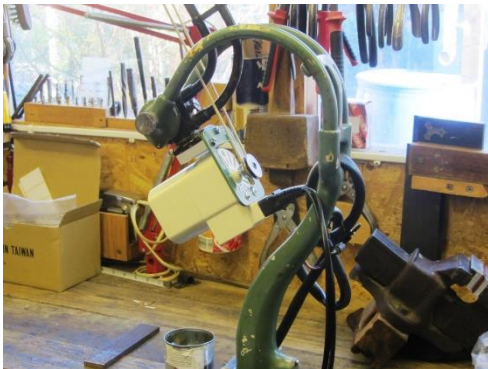
Motor assembly attached to drill arm mount
