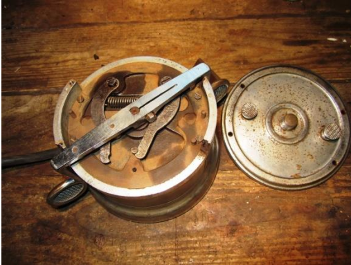
Foot control top showing return springs & levers
