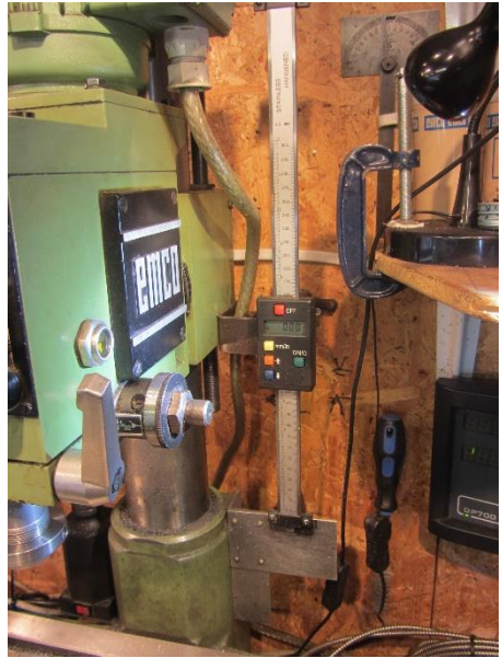
Figure 3. First Emco with retro-fitted z-axis
