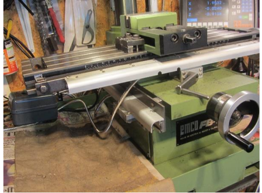
Figure 5. Machine-DRO x-axis under its protective cover. (The notches were a mistake)
