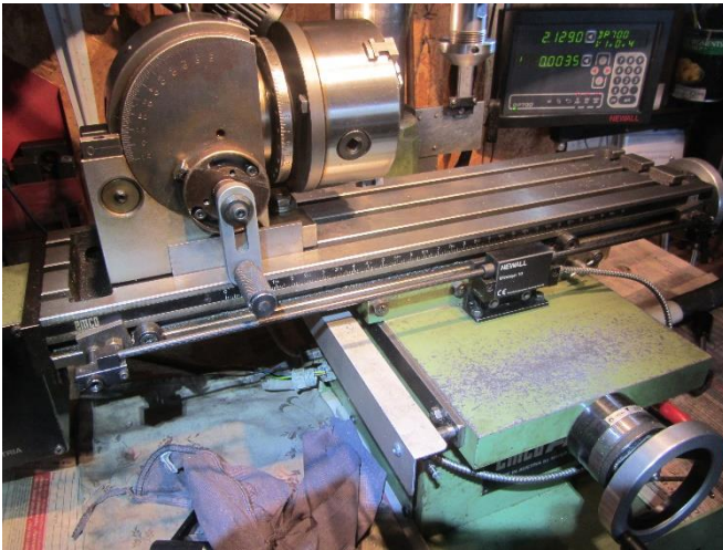
Figure 2. Newall scale & reader head on x-axis
