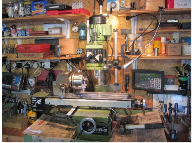
Figure 1. First Emco FB-2 with 2-axis Newall DRO
