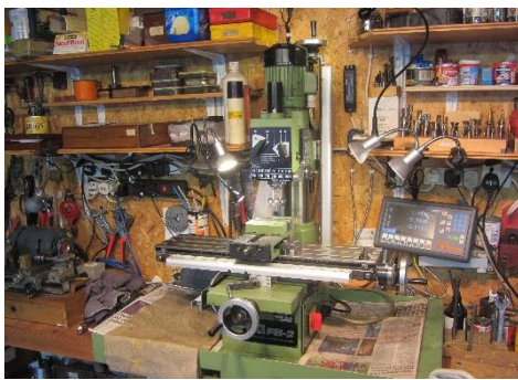
Figure 4. Second FB-2 with 3-axis Machine-DRO
