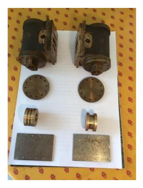
The cylinders come with front and rear covers and pistons but not the valve chests; two templates are provided to locate the drillings in new valve chest castings. The cylinder bore is 1.358" with a cylinder length of 3.125"
