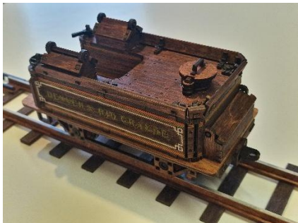
Rear of tender showing toolboxes, water filler port and flared tender top then with toolboxes and water filler port open
