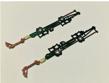
Locomotive frames with bearings fitted and front axle, eccentrics and valve gear
